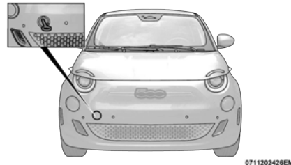
Front Tow Hook Installed
