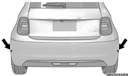
Radar Sensors Location
