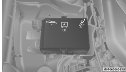
Front Power Distribution Center
