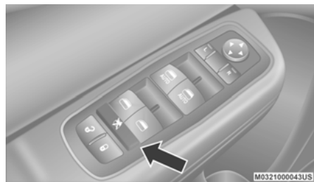
Window Lockout Switch
