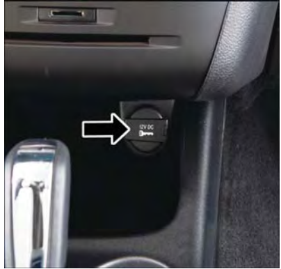
Front Power Outlet
