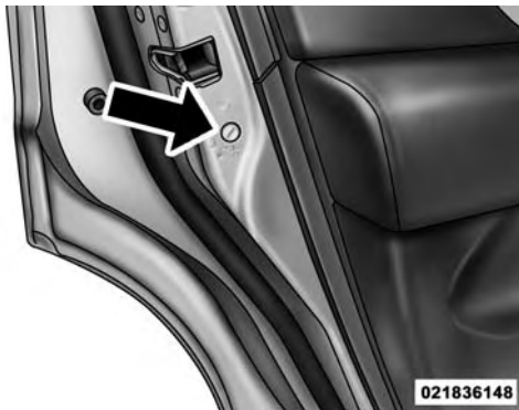
Child-Protection Door Lock Location
