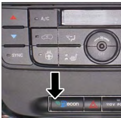
ECON Switch Location
