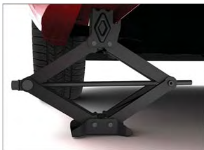
Rear Jacking Location Engaged
