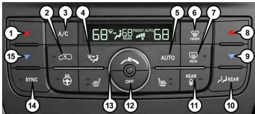
Three Zone Automatic Temperature Controls (ATC)
