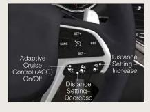
If the sensor does not detect a vehicle ahead of you, ACC will maintain a fixed set speed.
