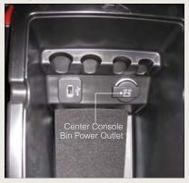
Power outlets are designed for accessory plugs only. Do not insert any other
