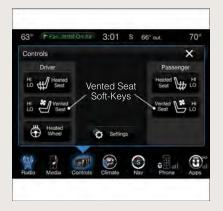
HIGH, press it a second time to choose LOW. Pressing the soft-key a third time will turn the ventilated seat OFF.
