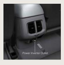
Watts, the power inverter may have to be reset manually. To reset the inverter manually, unplug the device and plug it in again. To avoid overloading the circuit, check the power ratings on electrical devices prior to using the inverter.
