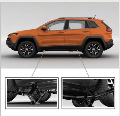
4. For the front tires, place the jack on the body flange just behind the front tire as indicated by the triangular lift point symbol on the sill molding.
