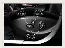
The power lumbar switch controls the amount of lumbar support needed. Push the switch forward to increase the lumbar support. Push the switch rearward to decrease the lumbar support. Pushing upward or downward on the switch will raise and lower the position of the support.
