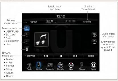
The iPod®/CD/AUX controls are accessed by touching the desired soft-key displayed on the side of the screen and choose between Disc, AUX, iPod®, Bluetooth® or SD Card.
