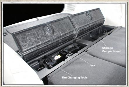
The scissor-type jack and tire changing tools are located in the passenger side compartment, behind the second row seat.
